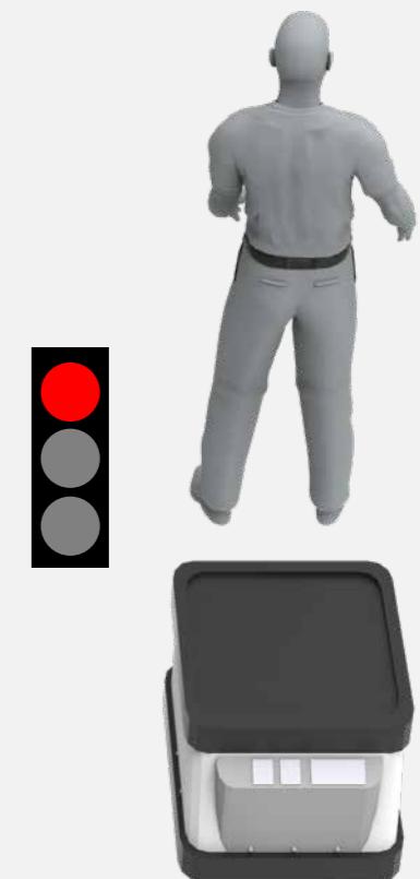
AGVs Stop and wait when there is an obstacle (e.g. a person).
