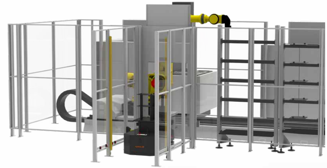
Transformer 6-axis: AMR with tray and lifter at a loading/unloading station.
