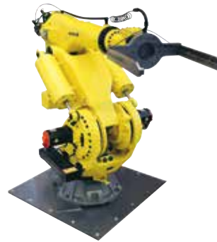
Automation – with 6-axis industrial robot
