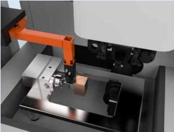
WorkPal 1 Application example: B-axis for Wire-cutting EDM (wire EDM).
